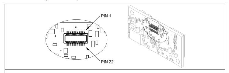
Figure 33. Decode Board Interface Connector
